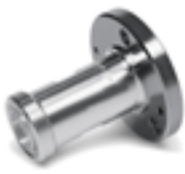
78EIA-716F Coaxial Adapter 7/8" EIA - 7-16 female
