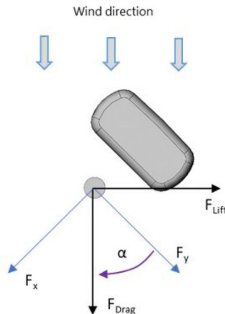
Figure 8: Reference frames (antenna vs wind tunnel)
