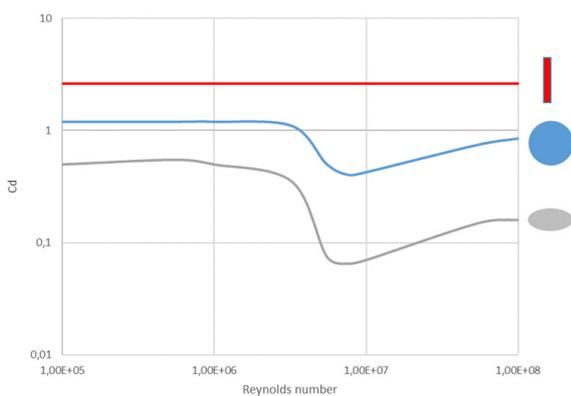
Figure 3: Drag coefficient vs Reynolds number
