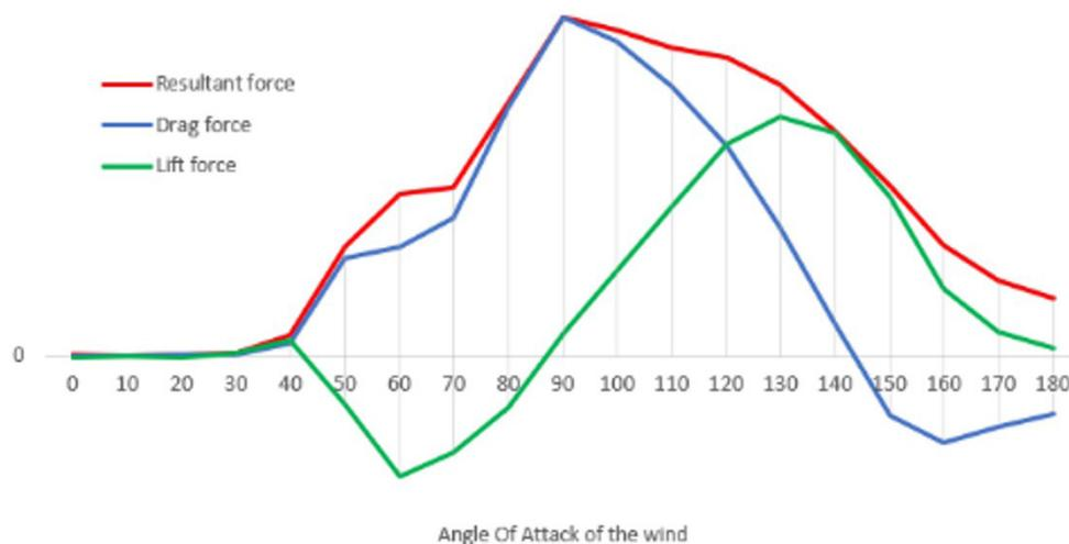
Figure 12: Drag, Lift and Resultant of the pole
