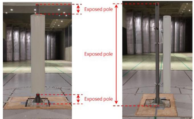
Figure 9: Subtraction when the pole is exposed
