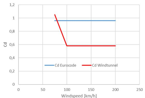
Figure 4: Comparison drag coefficient vs windspeed
