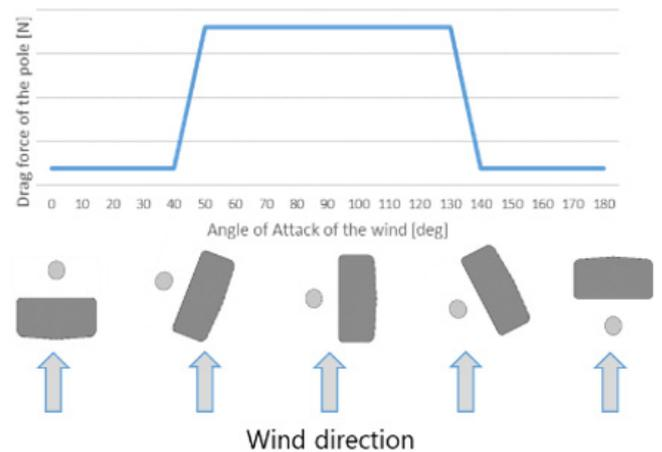
Figure 10: Drag of the pole depending on the angle
