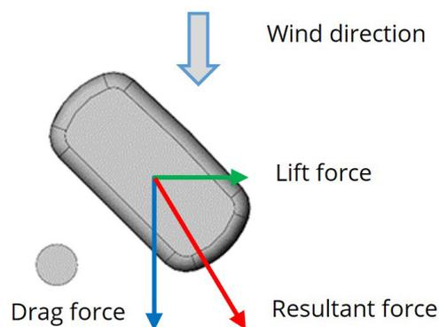
Figure 2: Drag, Lift and Resultant force
