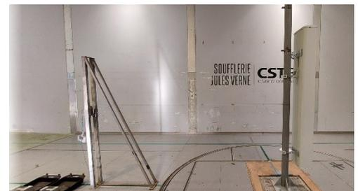
Figure 13: Calibration of the aerodynamic balance
