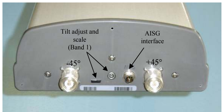
Figure 20: Single Band Antenna with connections labelled
