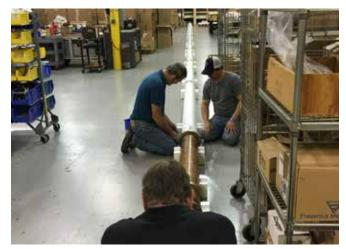
Testing 7 3/16" transmission line at the Myat Plant
