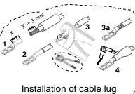
Installation of cable lug (if not factory fixed) with suitable crimp tool.
