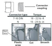
Wrap the connection with a layer of 3/4 (19mm) plastic tape, starting at 1" (25mm) from the connector or plastic strain relief of a jumper. Overlap the tape to half-width and jumper. extend the wrapping to the flange of the antenna connector. Avoid making creases or wrinkles. Smooth the tape edges
