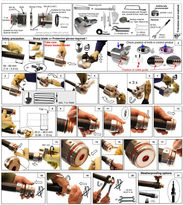
Additional weatherproofing must be used for Lite (Aluminium) cable types, a heat shrink sleeve with adhesive lining must be used for & RCF cables.
