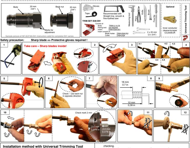
Attention: Trimming Tool to be handled and used with great care, blades are extremely sharp! It is recommended to use protective gloves. Do not use great force. Please refer to the instruction of the tool in addition! Keep the cable end downwards in order to prevent particles from entering during preparation.
