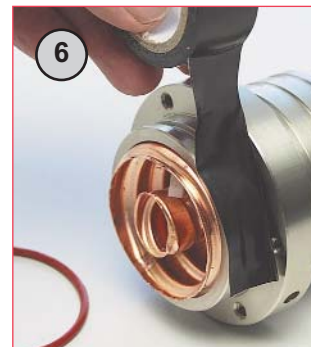
Remove O ring and protect groove with PVC tape.
