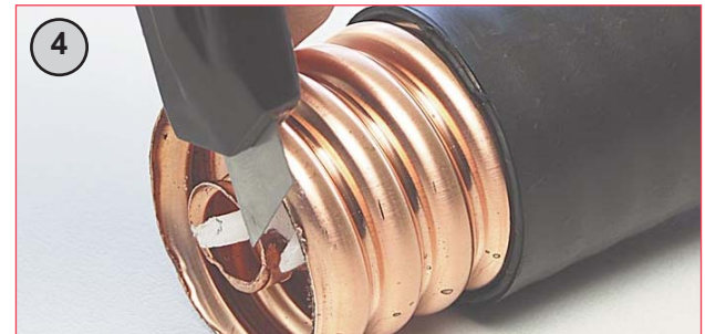
Trim and discard 5mm (3/16") off the helix then push back into original position. Make sure copper inner & outer edges are smooth and free of burrs and copper surfaces are clean, using the file and scouring pad. Ensure all debris is removed.
