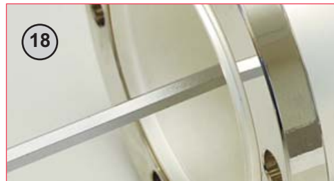
18 Tighten inner screw (clockwise) with 6mm hex key. Torque to 20Nm. Note: Copper washer (on the inner screw) is single use only. In case of repeated assembly replace used copper washer with the spare provided.
