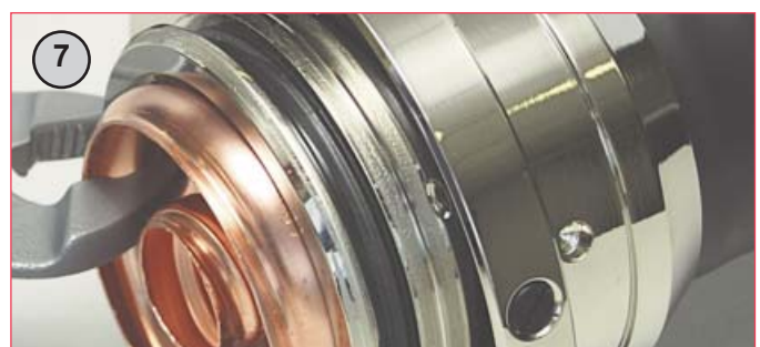
7 Flare outer conductor with soft jaw pliers. Work slowly around the perimeter flaring a small amount each time. Do not split the copper (refer Step 15 for remedial process).
