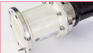
18 Tighten inner screw (clockwise) with 6mm hex key. Torque to 20Nm. Note: Copper washer (on the inner screw) is single use only. In case of repeated assembly replace used copper washer with the spare provided.
