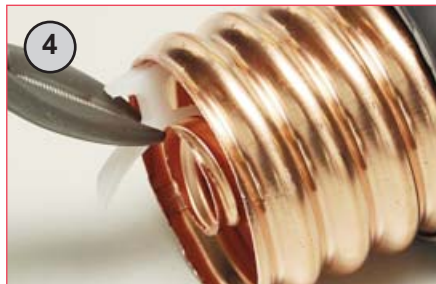
3 Pull out approximately 20mm (3/4") of helix. Trim and discard 12mm (1/2") off the helix then push back into original position. Make sure copper inner & outer edges are smooth and free of burrs and copper surfaces are clean, using the file and scouring pad. Ensure all debris is removed.
