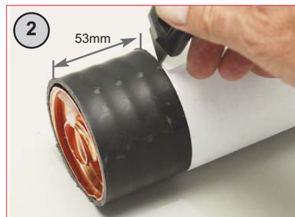
2 Trim jacket 53 mm (2.08"), ensure copper outer is not scored or cut. NB: A piece of paper makes a handy guide. JB Series cables only. Remove "Polymert" using white spirits, cloth and scouring pad until copper is clean.
