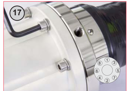
17 Tighten the connector body screws following the sequence shown (inset) then torque to 8Nm. Repeat tightening process.
