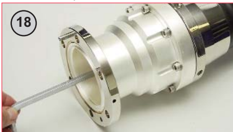
Tighten inner screw (clockwise) with 8mm hex key. Torque to 30Nm approx. Note: Copper washer (on the inner screw) is single use only. In case of repeated assembly replace used copper washer with the spare provided.
