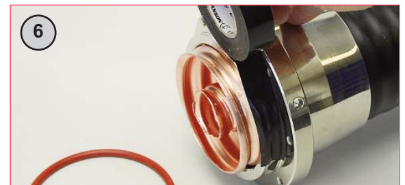
6 Remove O-ring and protect groove with PVC tape.
