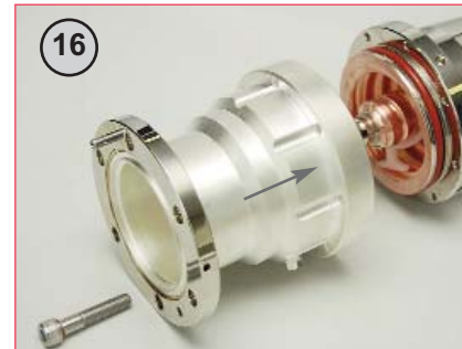
Lubricate and refit O-ring with silicone grease. Fit connector body.
