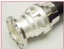
Tighten inner screw (clockwise) with 8mm hex key. Torque to 30Nm approx. Note: Copper washer (on the inner screw) is single use only. In case of repeated assembly replace used copper washer with the spare provided.
