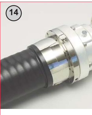
Gas Pass process: Using a 3mm 1/8" drill bit, drill a hole through the PTFE spacer midway between the inner assembly and the connector body.
