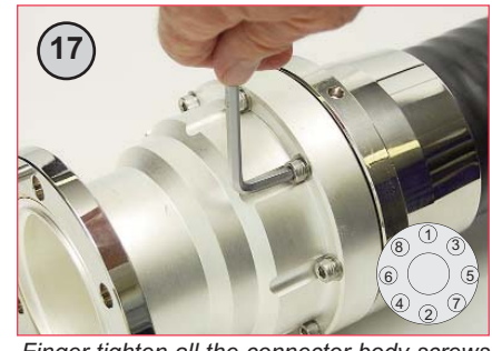
Finger tighten all the connector body screws clockwise following the sequence shown (inset) torque to 8Nm. Repeat tightening process
