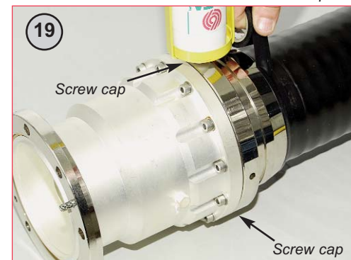
19 Remove both screw caps on back nut. Finely spray back nut/cable with water to accelerate curing. Inject sealing compound (approx 120cc) until the sealant appears at the opposite side of the back nut. Replace cap to stop further flow of sealant. Wrap insulating tape around the rear of the back nut/cable. Puncture the tape in 4 places as shown and then continue injecting compound until it appears at the puncture points. Remove sealant tube cartridge and replace screws. Do not pressurise for 24 hrs to allow compound to harden.
