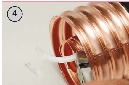
3 Pull out approximately 50mm (2.0") of helix. Trim and discard 40mm (1 1/2") off the helix then push back into original position. Make sure copper inner & outer edges are smooth and free of burrs and copper surfaces are clean, using the file and scouring pad. Ensure all debris is removed.
