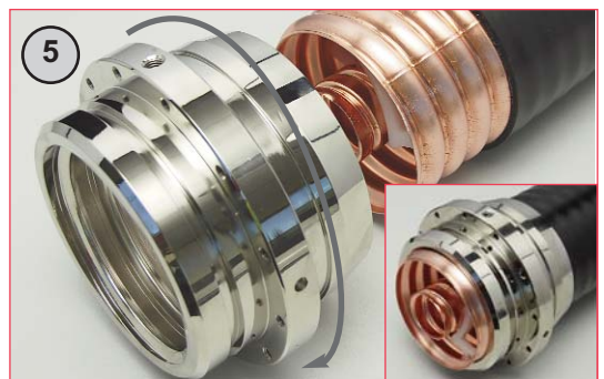
5 Screw connector back nut clockwise as far as possible onto the cable.
