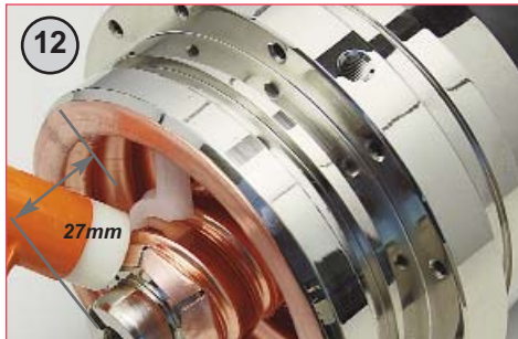
12 Screw inner cable piece out until it protrudes 27mm (1-1/16") from the outer conductor flared face. Hammer copper to form over inner cable piece. Clean assembly.
