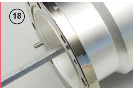
18 Tighten inner screw (clockwise) with 10mm hex key. Torque to 40Nm. Note: Copper washer (on the inner screw) is single use only. In case of repeated assembly replace used copper washer with the spare provided.
