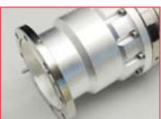
18 Tighten inner screw (clockwise) with 10mm hex key. Torque to 40Nm. Note: Copper washer (on the inner screw) is single use only. In case of repeated assembly replace used copper washer with the spare provided.
