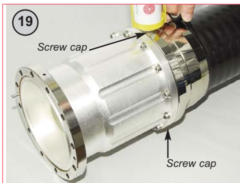
19 Remove both screw caps on back nut. Finely spray back nut/cable with water to accelerate curing. Inject sealing compound (approx 250cc) until the sealant appears at the opposite side of the back nut. Replace cap to stop further flow of sealant. Wrap insulating tape around the rear of the back nut/cable. Puncture the tape in 4 places as shown and then continue injecting compound until it appears at the puncture points. Remove sealant tube cartridge and replace screws. Do not pressurise for 24 hrs to allow compound to harden.
