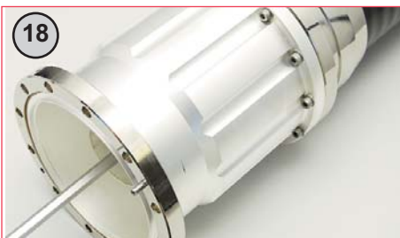
18 Tighten inner screw (clockwise) with 14mm hex key. Torque to 60Nm. Note: Copper washer (on inner screw is single us. In case of repeated assembly replace used copper washer with spare provided.
