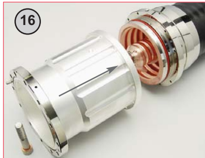
16 Do not use dirty or damaged O-rings. Apply silicone grease to O-ring. Place O-ring in position on back nut. Fit connector body.
