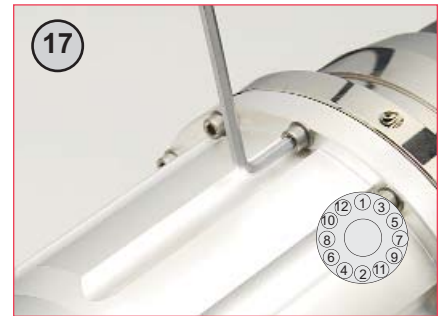
17 Tighten connector body screws following the sequence shown (inset) then torque to 8Nm. Repeat tightening process.
