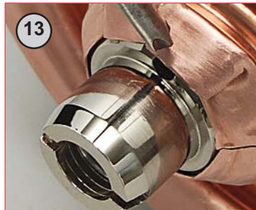
13 Indent cable inner conductor to prevent connector inner nut from rotating.
