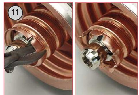
11 Snip inner conductor with 4mm wide x 6mm deep V cut, approx every 15mm.
