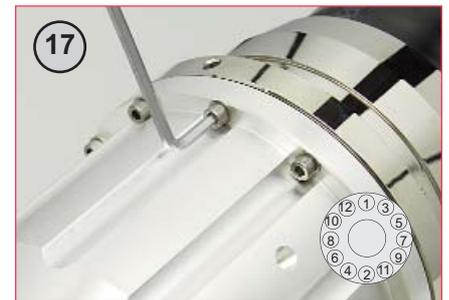
17 Finger tighten all the connector body screws then following the sequence shown (inset) torque to 8Nm. Repeat the sequence.
