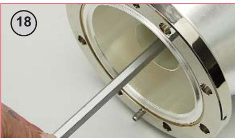
18 Tighten inner screw (clockwise) with 14mm hex key. Torque to 60Nm. Note: Copper washer (on the inner screw) is single use only. In case of repeated assembly replace used copper washer with the spare provided.
