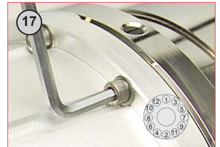
17 Finger tighten all the connector body screws then following the sequence shown (inset) torque to 8Nm. Repeat tightening process.
