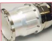
18 Tighten inner screw (clockwise) with 14mm hex key. Torque to 60Nm approx. Note: Copper washer (on the inner screw) is single use only. In case of repeated assembly replace used copper washer with the spare provided.
