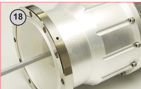
18 Tighten inner screw (clockwise) with 14mm hex key. Torque to 60Nm approx. Note: Copper washer (on the inner screw) is single use only. In case of repeated assembly replace used copper washer with the spare provided.
