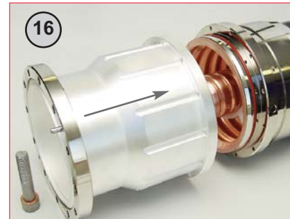
16 Do not use dirty or damaged O-rings. Apply silicone grease to O-ring. Place O-ring in position on back nut. Fit connector body.
