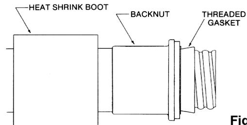
6. Slide the backnut forward as far as possible over the threaded gasket. Assemble the insert plate with screws to the face of the backnut, compressing the threaded gasket. See Figure 4.
