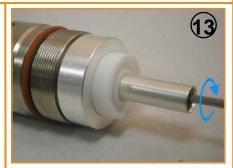
Insert inner cable assembly into back nut and finger tighten using M3 hex key.
