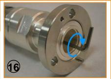
Re-tighten inner assembly to a torque of 2.6 Nm.
