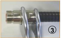
Tighten the threaded bushing to the back nut with 32 mm spanners as shown
