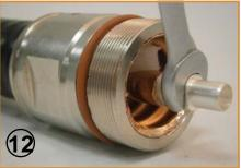
Screw inner pin into the cable inner conductor and tighten using the M7 spanner .
