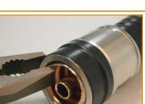
Remove the O-ring and protect the groove with a piece of the earlier removed jacket and PVC tape. Flare outer conductor with soft jaw pliers to avoid splitting or deep scratches.
