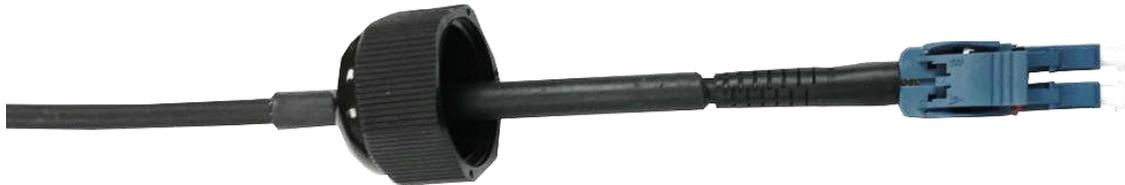
Carefully feed compression nut over fiber jumper connector and slide onto jacketing. Do not twist or bend the LC connector or fiber. Excessive force or bending may break the fiber or connector components.
