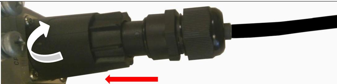
Slide the FullAXS compatible sleeve up to the RRH. Turn top nut clockwise to secure to RRH bulkhead connector.
