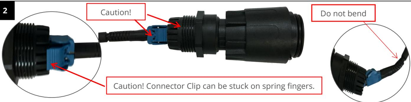
Feed the fiber connector into the sleeve until the Connector comes out. **Caution: do not apply too much force as doing so can cause damage to the fiber and gland spring fingers.**
