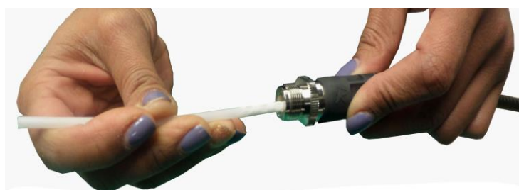
Cleaning ODC socket using the 1.25mm one-click cleaner
