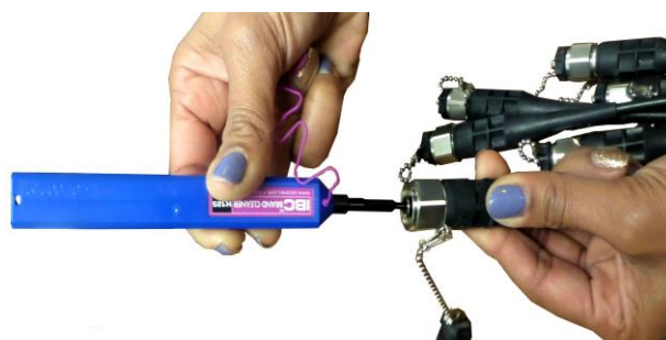
Cleaning ODC plug using the one-click cleaner
