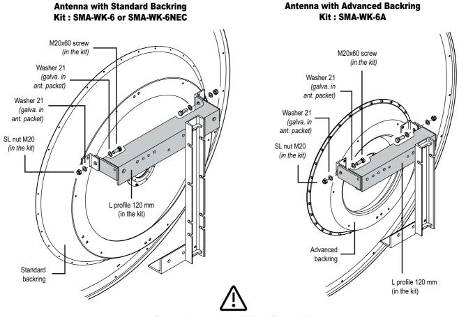
Do not use the galvanized steel M20 nuts, SL washers 20 and screws M20x60 provided with the antenna
