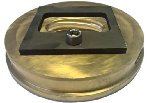
Picture shows flanging die for E65 waveguide
