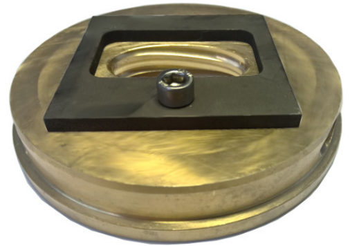
Picture shows flanging die for E65 waveguide
