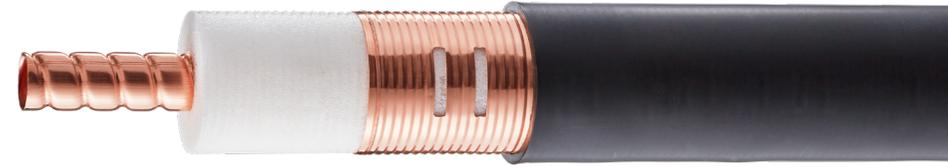
RFS RADIAFLEX® radiating cable is the world’s leading “leaky feeder” cable solution. It is designed to deliver contoured indoor RF coverage with radio signals leaked from the apertures on the radiating cable’s outer conductor. This allows network operators to provide scalable and practical broadband wireless services for confined areas, such as tunnels, mines and large building complexes.
