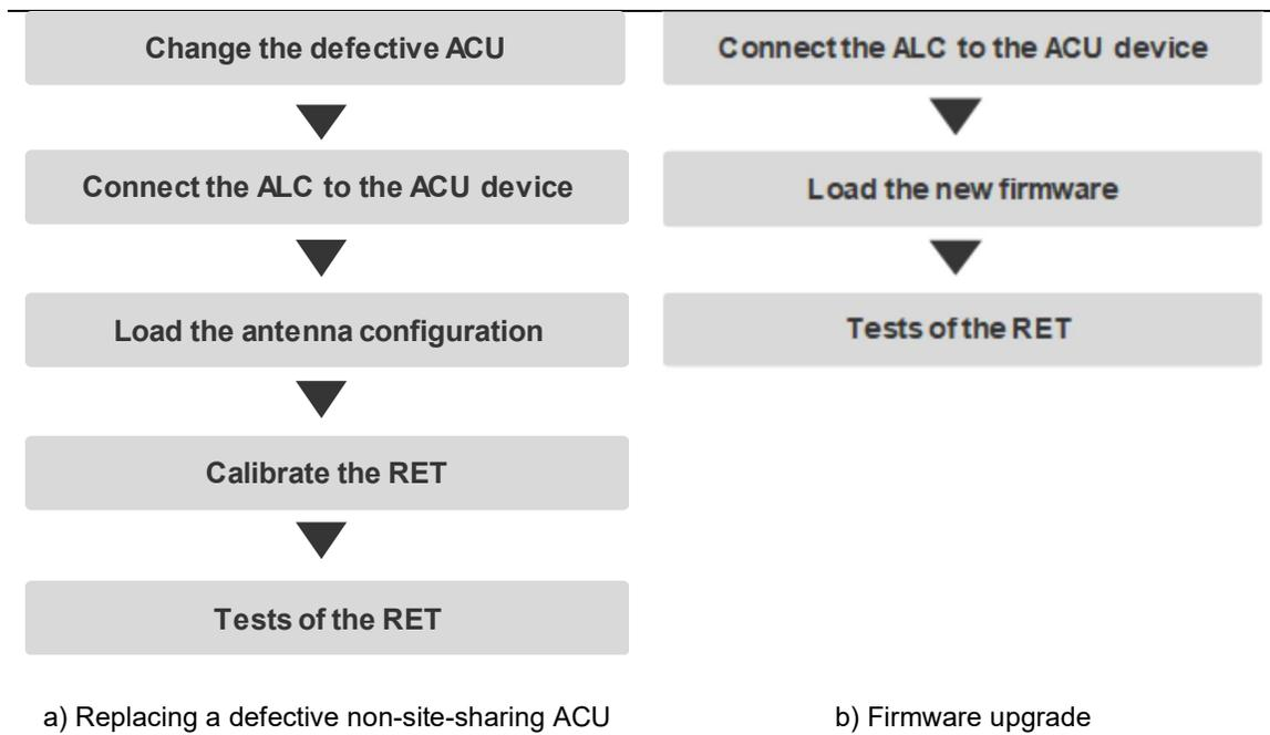
**Figure 1:** Flowchart for maintaining a non-site-sharing ACU
