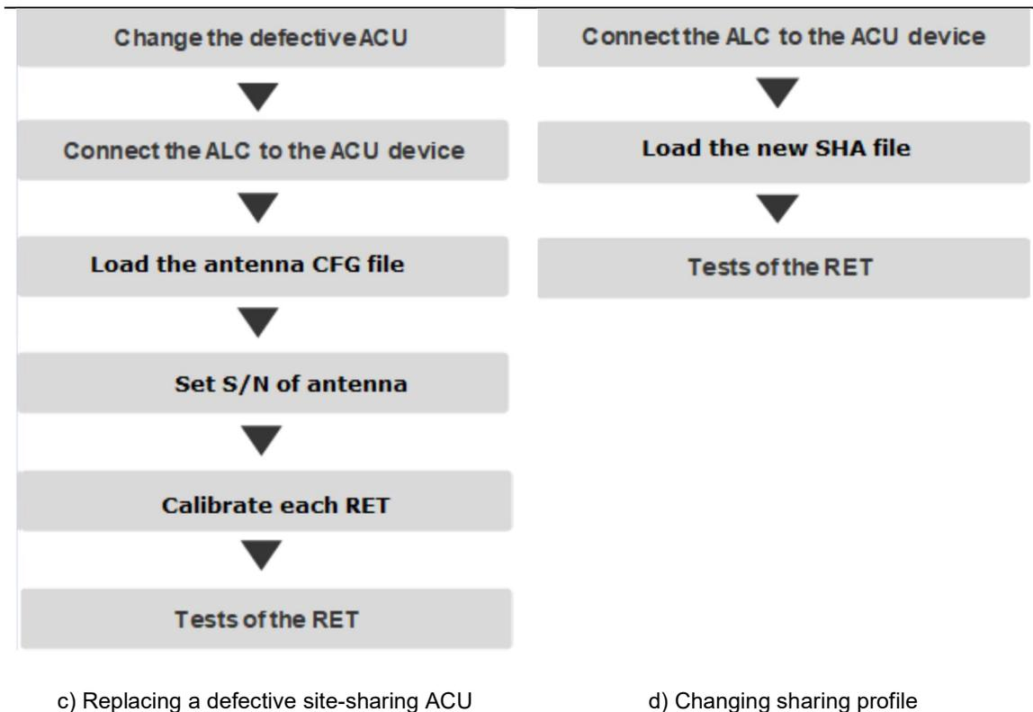
**Figure 1:** Flowchart for maintaining a site-sharing ACU
