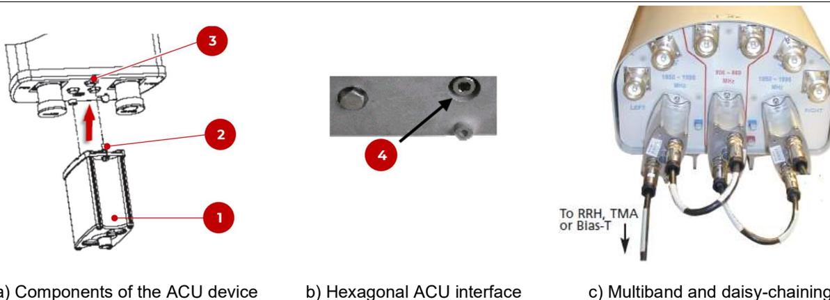
**Figure 2:** Steps for replacing an ACU-A20 device
