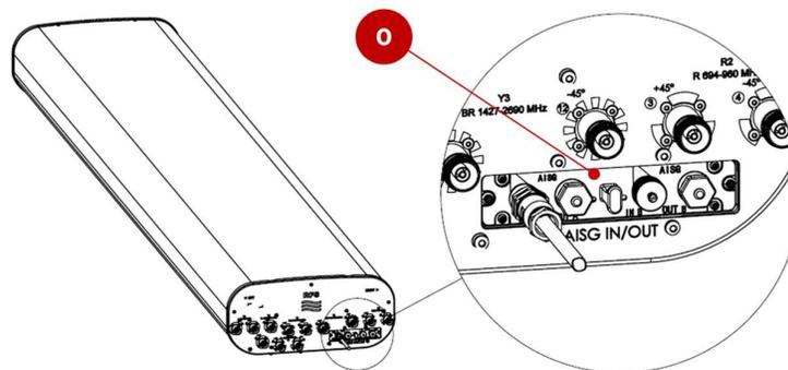
**Figure 3:** Location of the ACU on an antenna
