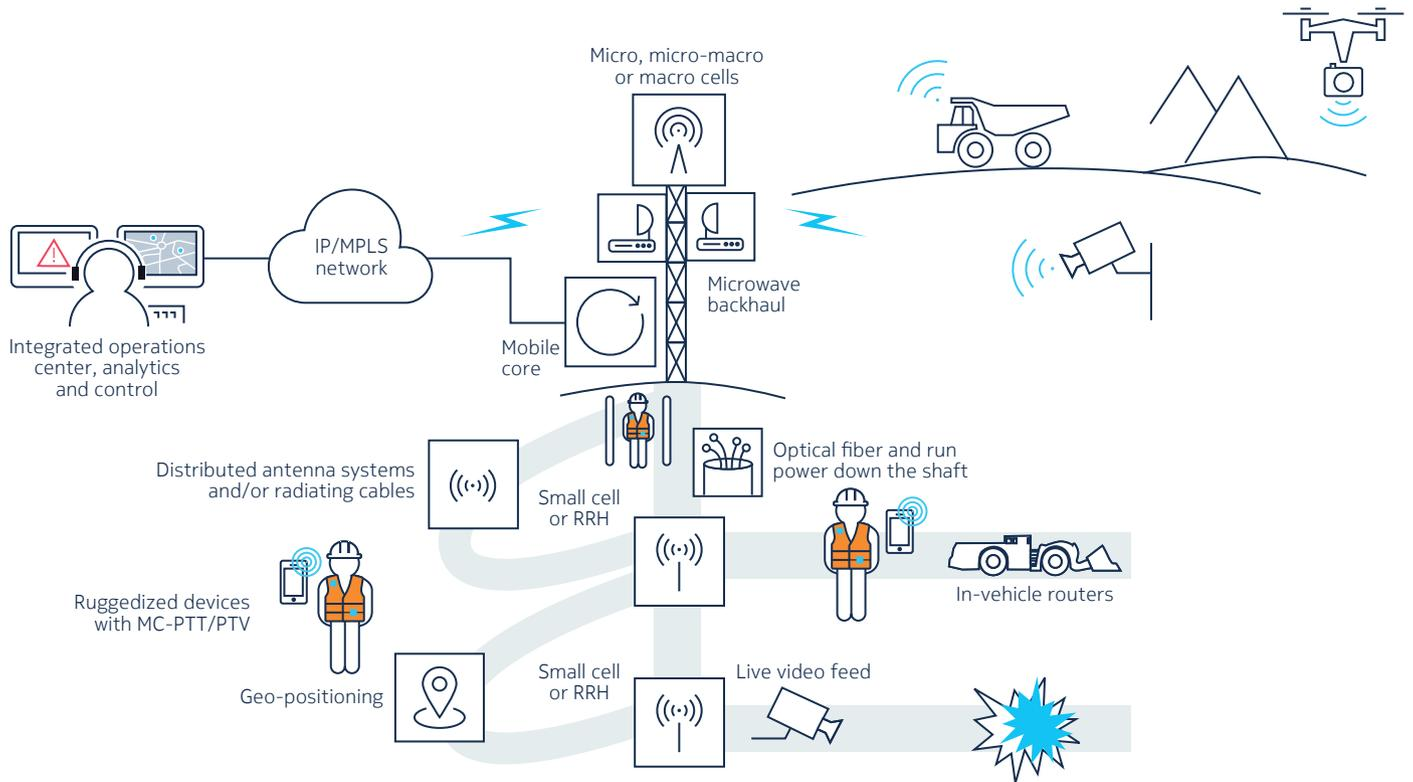
To ensure flexible coverage, the network may need a combination of radio technologies such as small cells, micro remote radio heads (RRHs), radiating cables (also known as leaky feeders) and distributed antenna systems (DASs), all of which need to be integrated with existing UHF/VHF systems. Table 2 shows a comparison of radio access network (RAN) architecture options that use different combinations of radio technologies.
