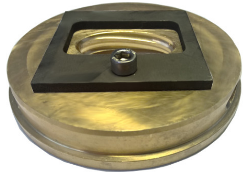
Picture shows flanging die for E65 waveguide
