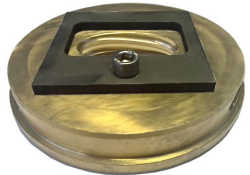
Picture shows flanging die for E65 waveguide
