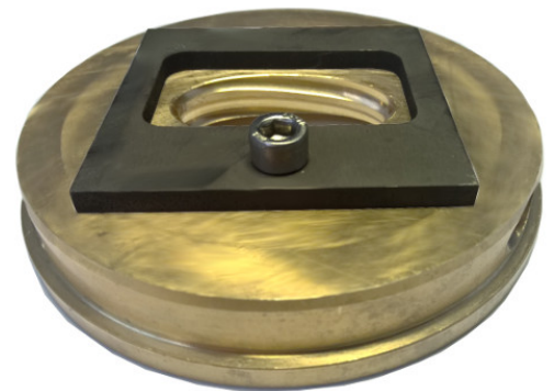
Picture shows flanging die for E65 waveguide
