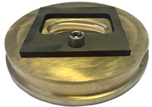
Picture shows flanging die for E65 waveguide
