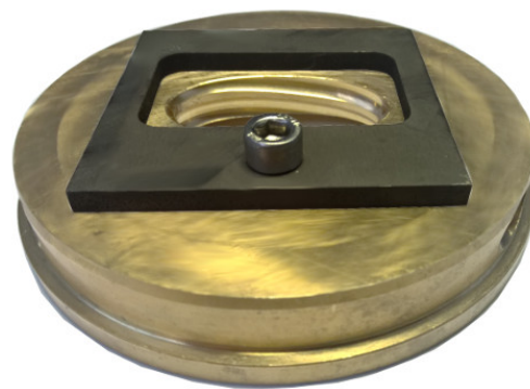
Picture shows flanging die for E65 waveguide
