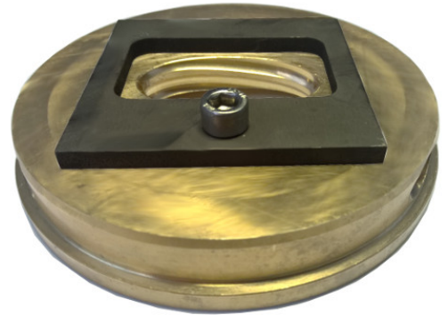
Picture shows flanging die for E65 waveguide
