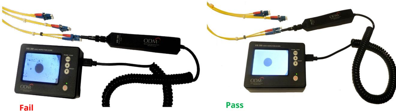
**Important Note:** In the event of failure, clean connectors as shown below, refer to optical fiber cleaning section within this document for additional cleaning suggestions.
