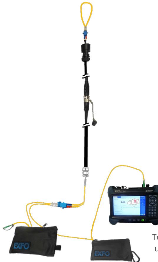
Test diagram using OTDR device
