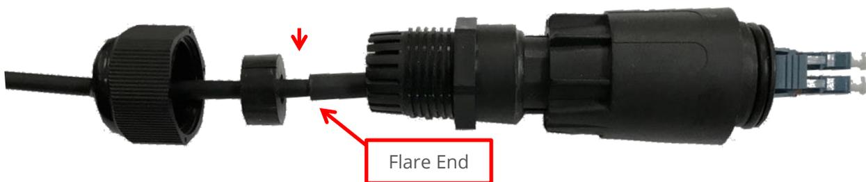
Wrap the rubber split grommet around the jacketing and VERY CAREFULLY push it UNDER the clamping fingers until the grommet is flush with the finger ends. **Caution: it will be necessary to gently lift the fingers.**
