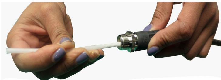
Clean the ODC socket using the Swab stick, gently moisten the cleaning swab tip with an alcohol or Electro-Wash pen wet solution and gently clean each connector
