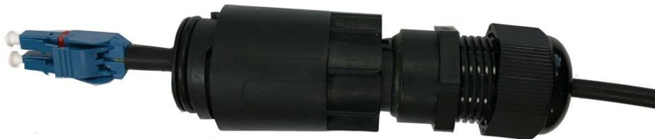
Slide FullAXS compatible gland body down jacketing to allow access to the fiber end connector. Do not pull the fiber end connector through the sleeve or damage may occur.
