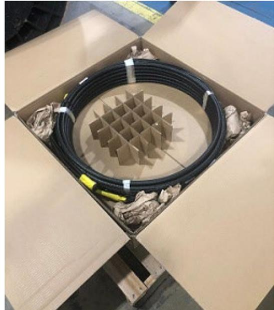
Top and bottom assembly terminations will be protected and identifiable. See example below:
