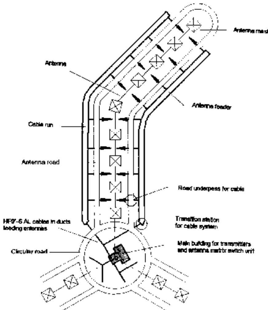
Fig. 1: Schematic Representation of the Wertachtal Transmitting Center
