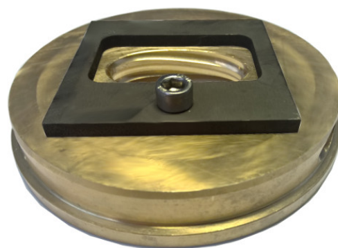
Picture shows flanging die for E65 waveguide
